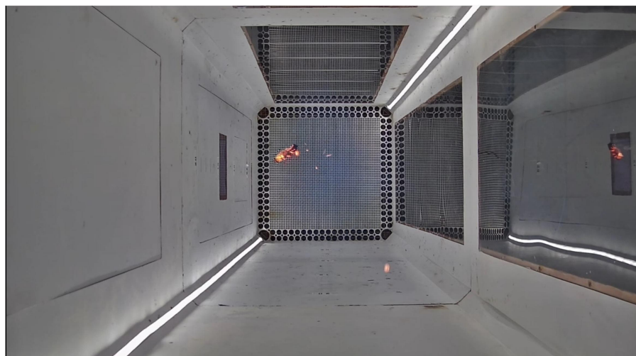
Fig. 3. A video frame from the top-view camera showing a burning bark sample illustrates the challenges posed by changes in bark shape and colour, small fragments broken off from the main bark and reflection from the side window during combustion.
