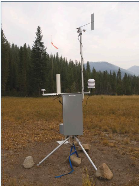
A remote, automatic weather station collects weather data during a fire. This information is incorporated in near-real time to the models that feed the Hot-Dry-Windy Index.
