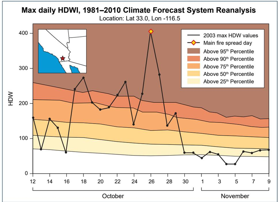
An example of output from the Hot-Dry-Windy Index (HDWI) for the 2003 Cedar Fire in southern California. From the interactive website, users can select a location in North America and see the HDWI values for the past 10 days and the forecast for the next 7 days. A high spike indicates a bad fire weather day. Adapted from McDonald et al. 2018.
