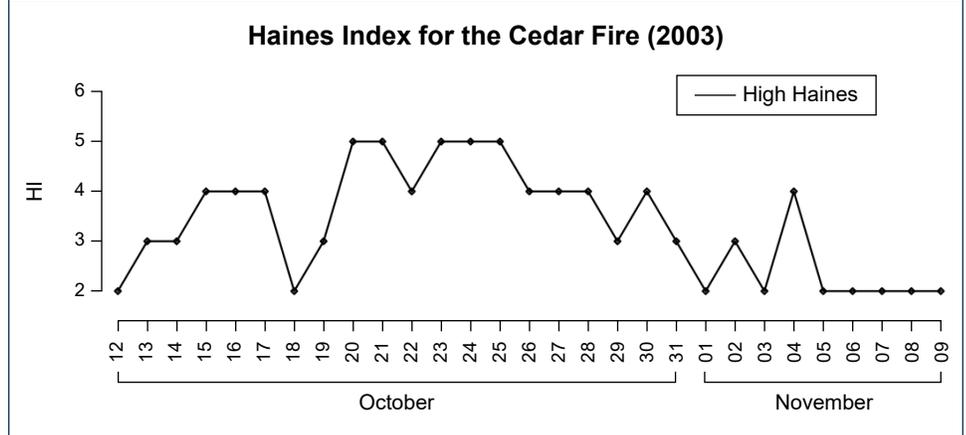
The spike in Hot-Dry-Windy Index (HDWI) coincides with the big growth event on the 2003 Cedar Fire. In contrast, the Haines Index was higher on days of more moderate growth and dropped on the big growth day. Adapted from Srock et al. 2018.
