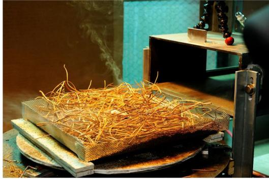
**Figure 1. The fuel sample holder was made of wire mesh and was supported 1.3 cm above the weighing platform by strips of cement board. The load cells can be seen underneath. The samples were placed at the outlet of a wind tunnel.**
