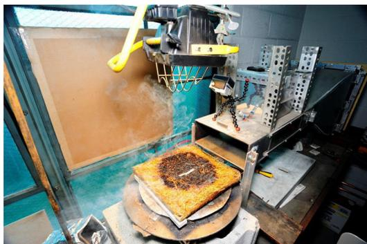
**Figure 2. A halogen work lamp was suspended above the fuel to mimic solar radiation. Here you can also see the GoPro camera and the whole of the wind tunnel.**
