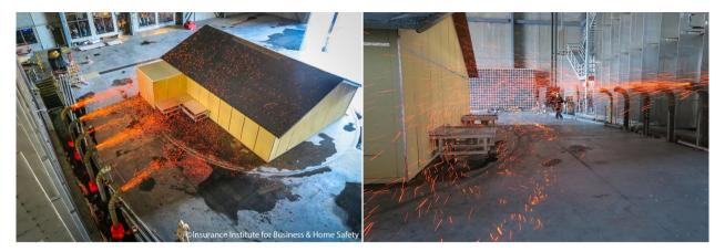
Fig. 4. Test building and ember generator system used in the accumulation study. As shown, (left) the collection trays were initially covered with a solid panel until steady flow from the generators was observed, at which point the covers were removed (right) allowing embers to land in the water-filled pans.
