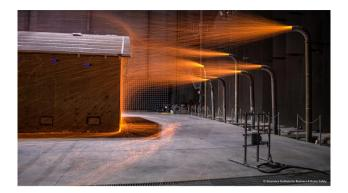
Fig. 8. As seen in testing conducted at the IBHS Research Center, with a smooth landing surface (concrete in this case), ember accumulation is greatest at the ground-to-wall intersection and at a stagnation point away from the building.
