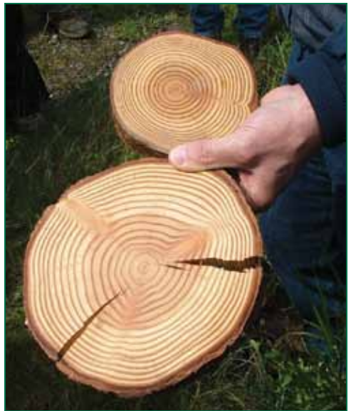
Figure 6. A comparison of cross-sections cut from healthy (bottom) and diseased (top) Douglas-fir trees of approximately the same age from different locations, demonstrating that growth loss can be severe and that wood density, earlywood to latewood ratio, and quality can be affected by Swiss needle cast.
